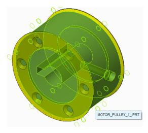
Fig.7 Isometric view of pulley showing the parallel keyway
