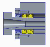
Fig. 5 sectional view of Morse taper, bearing, Lybrinth
