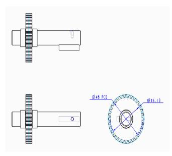
Fig.6 Detail drawing of shaft and gear
